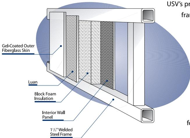
USV's products feature welded steel frames on gas- or diesel-powered chassis. High-gloss, imported fiberglass skin covers the vacuum-bonded, hard-wall body which is topped by a seamless, leak-proof rubber roof. Between the exterior walls and roof and vinyl interior wall paneling is sound-absorbing block-foam insulation.
